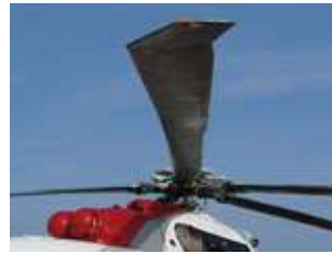
Composite main rotor blades
