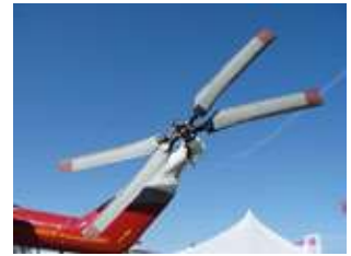
X-shaped tail rotor
