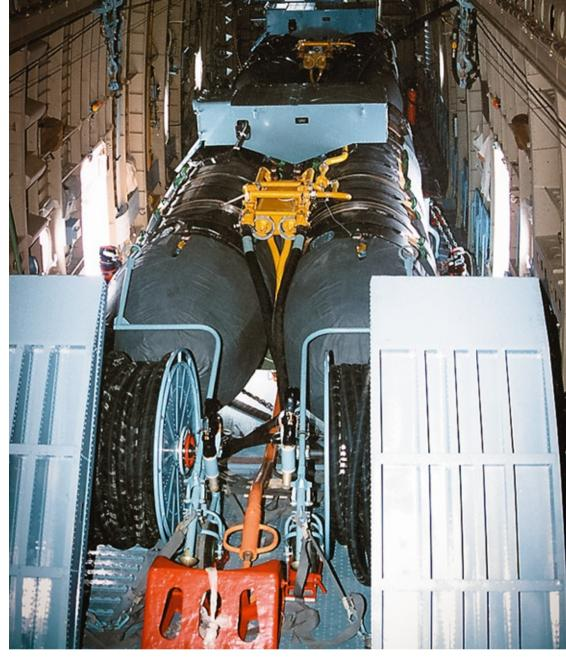
The refuelling version is designed for the transportation of different types of fuel (kerosene, diesel) and lubricants. The onboard equipment allows for autonomous refuelling both of aircraft and ground equipment.
