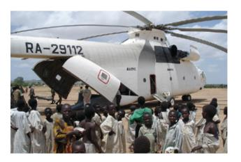
The Mi-26T2 is capable of transporting up to 82 persons for the distance of 800 km. This capability makes the aircraft irreplaceable in case of urgent evacuation of people from an emergency situation. For transportation of people the helicopter can be equipped with 82 removable light-weight seats.
