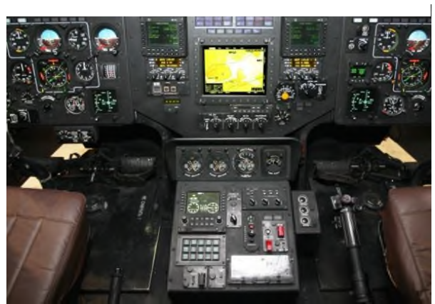
Cockpit adaptation for using NVG
