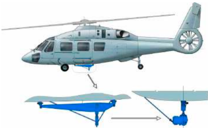
7.7 Attachment of cargo at the external sling
