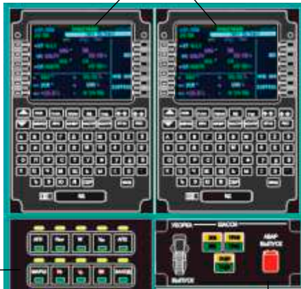
Control panel for landing gear retraction / extension / emergency extension
