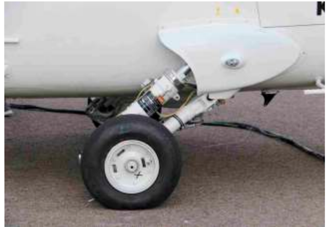
3.3 Wheel landing gear with increased shock absorbing capability
