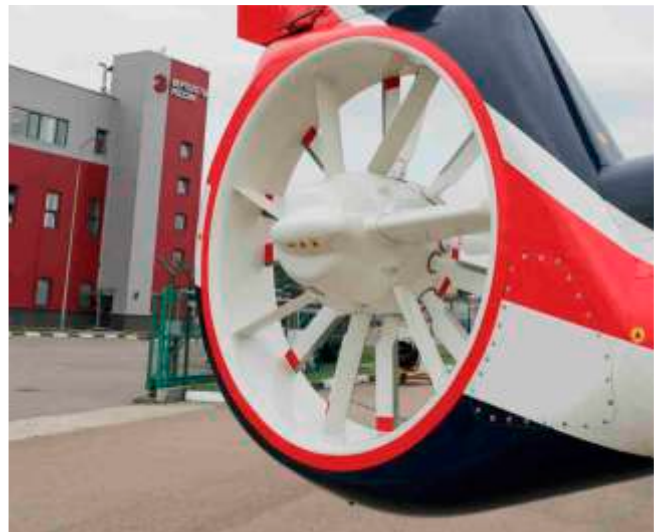
3.4 Fan-in-fin tail rotor
