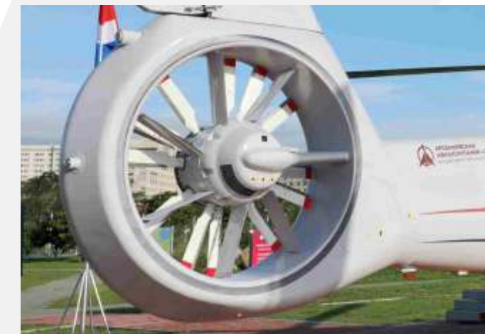
Fan-in-fin 12-blade tail rotor
